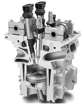
Fig. 1 Cross section view of the N53 engine 10)
