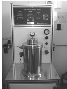
Fig. 6 Pressure drop test equipment
