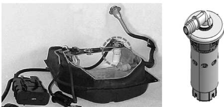
Fig. 1 Vent valve in the fuel system
