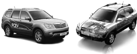
Fig. 3 Fuel cell system package layout of Tucson FCEV in Hyundai Motor Co.
