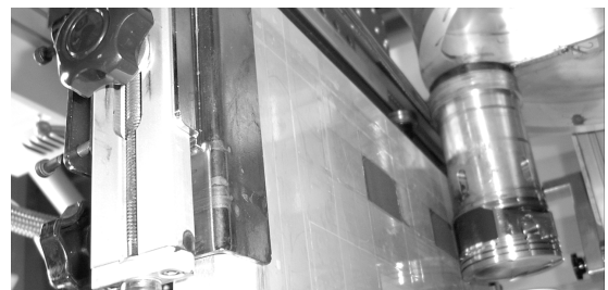
(b) Piston and rotating jig for fixing a piston (lower side)
