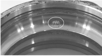
Photo. 1 Flaking of hub bearing outer
