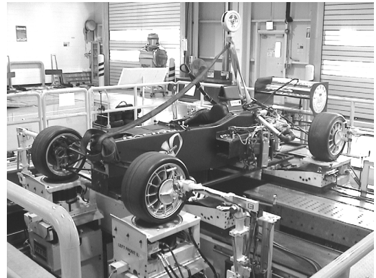
Photo 1 The kinematic test of the PACE vehicle
