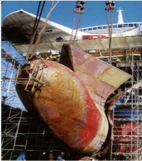
Fig. 4. The scene of bulbous bow conversion. 자료출처: Delta Marine Report, 2005.
