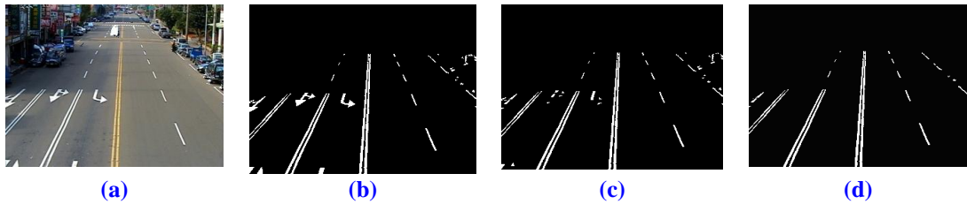
Fig. 7. Examples of removing horizontal and vertical noise. (a) Original background image. (b) A binary image before removing noise. (c) A binary image after removing horizontal noise. (d) A binary image after removing vertical noise.
