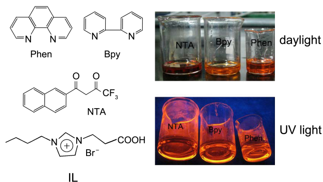
Figure 1. The Ionic liquid (IL), organic ligand and the photographs of europium-containing ionic liquids.
