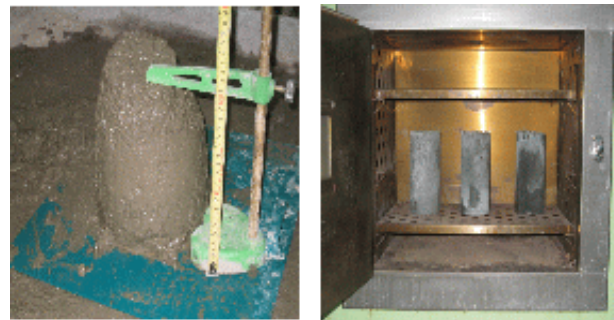
(a) Slump test
