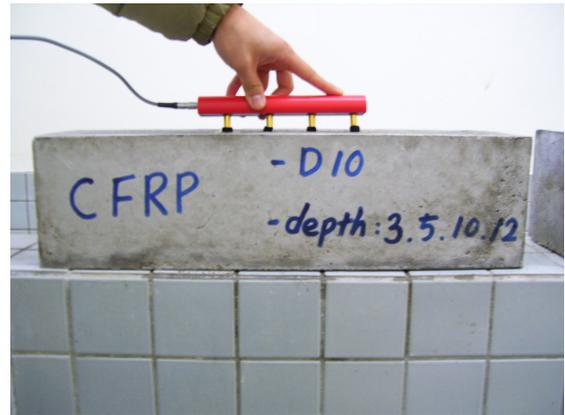
Photo 4 Measurement of surface resistivity
