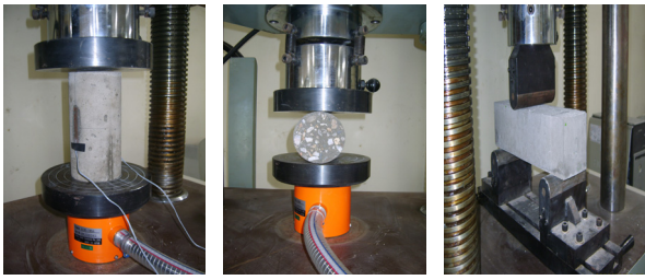
(a) Compressive strength and elastic modulus (b) Tensile strength (c) Flexural strength
