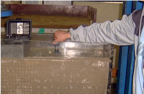
Photo 4 Measurement of undrained shear strength on the surface
