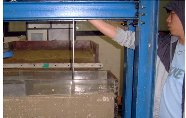
Photo 5 Measurement of undrained shear strength in the soft soil layer
