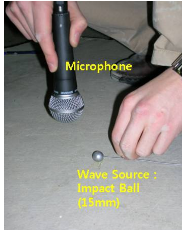
Fig. 3 Testing Configuration of Contactless Impact-Echo Sensing
