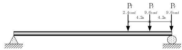
Fig. 5 Truck wheel loading on a longitudinal section
