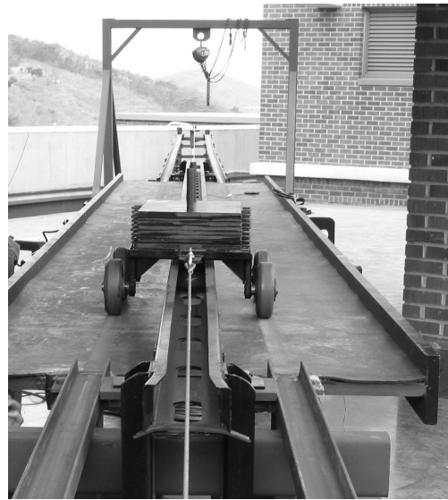
Fig. 3 Laboratory setup for moving vehicle tests
