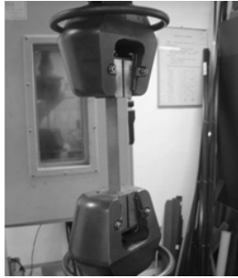
Fig. 2 View of Mechanical property test (AFRP)
