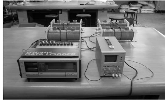
Fig. 2 View of Chloride Diffusion Test
