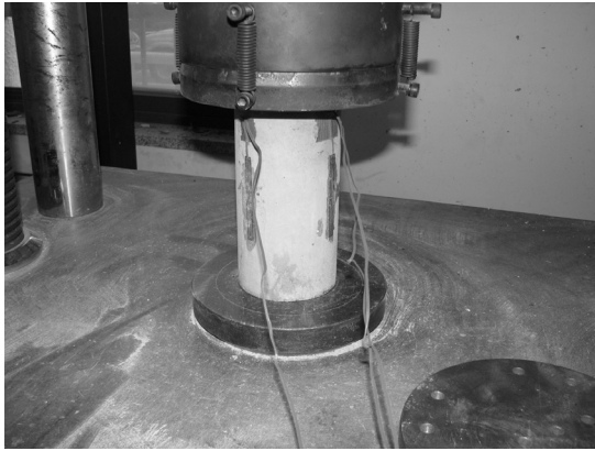
Photo 1 Test figure of compressive strength specimen
