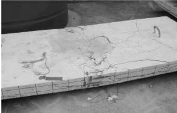
Photo 3 Breaking figure of flexural test
