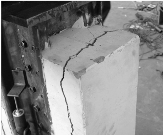
Photo 2 Breaking figure of Push-Out Test
