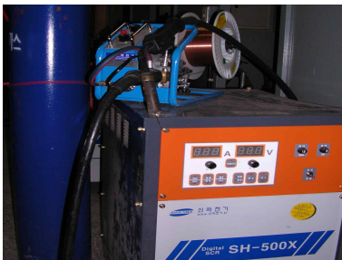
(a) CO 2 Welding machine
