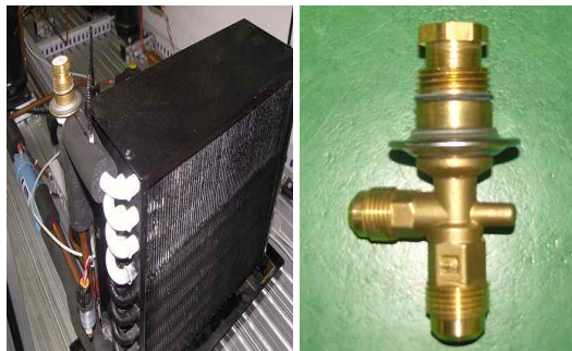
Fig. 6. photo of manual expansion valve.
