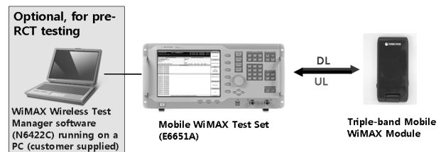
Fig. 8. Diagram of triple-band mobile WiMAX transceiver module Test.
