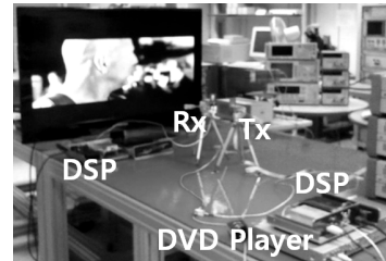
Fig. 9. Demonstration of the wireless video transmission using the fabricated LTCC SiP transmitter and receiver modules.
