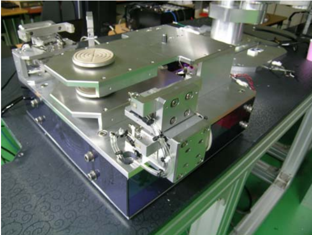
Fig. 7 A prealigner constructed for experiment
