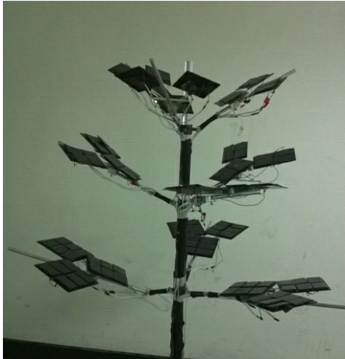
Fig. 4. Photograph for the tree-mimic installation of the solar cell modules.
