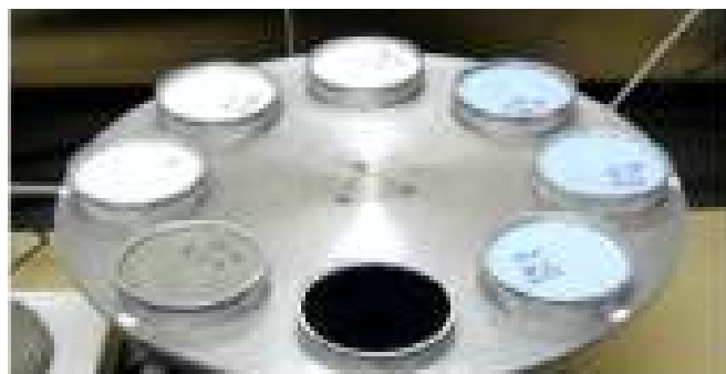
<Fig. 1> Moisture vapor test – Open cup testing instrument.
