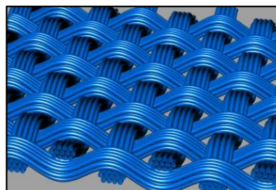
<Figure 1> Perspective view of a woven fabric model showing intersections of warp and filling yarns, friction-causing element during initial bending of a fabric (plain weave structure of multi-filament yarns)
