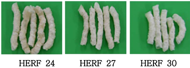
Fig. 1. Shapes of rice extrudates with different moisture contents 24, 27, and 30%.
