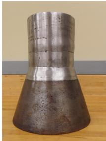
Fig. 2 Photograph of pressurizer spray nozzle test specimen
