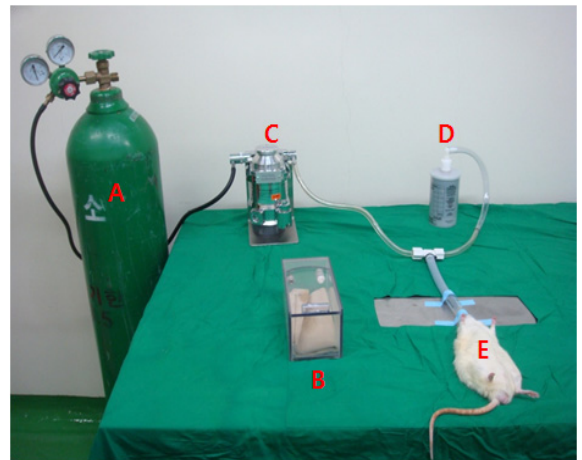
Fig. 1. Device setup for rodent anesthesia(A. Oxygen, B. Anesthesia induction chamber, C. Vaporizer, D. Device for anesthetic gas removal, E. Animal for surgery)
