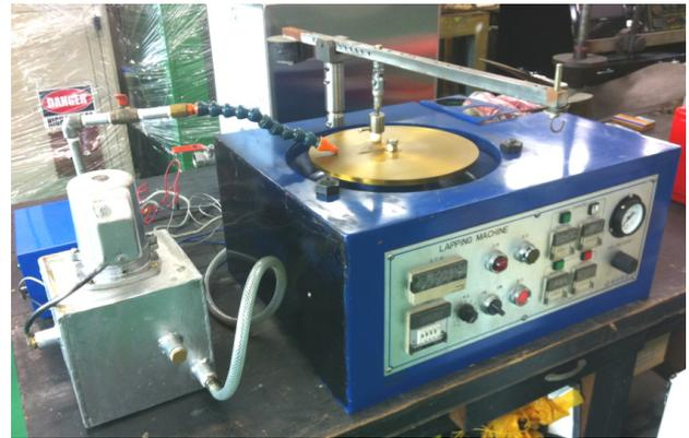
Fig. 3 Pin on disk system of friction and wear test apparatus
