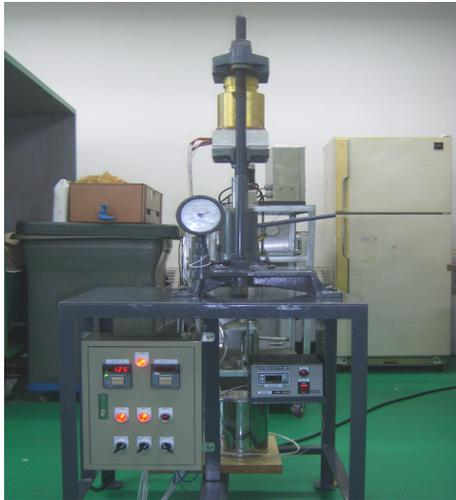
Fig. 1 Compression apparatus for porous PTFE composite.
