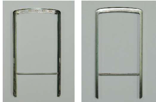
Fig.12 Metal front case for mobile phone assembled with reinforcement by welding process
