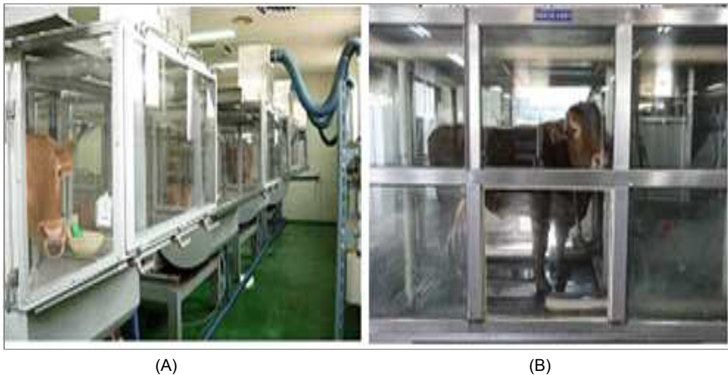
Fig. 8. Respiration chamber facility practices at National Institute of Animal Science.
