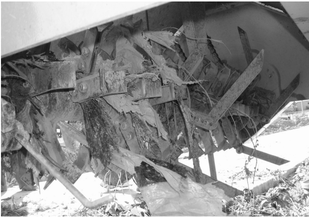
Fig. 10 View of the mulching vinyl and vines caught in vine crushing part.
