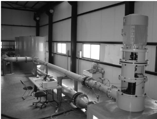
Fig. 7 RCP test loop at KIMM
