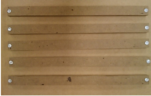
Fig. 1. Typical examples of green tea - wood fiber hybrid board specimens for flexural vibration test (20 mm (W) x 12 mm (T) x 300 mm (L)).
