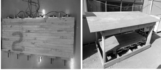
Fig. 3. Specimens for measuring compressive performance of stress-laminated timber (left: indoor, right: outdoor).
