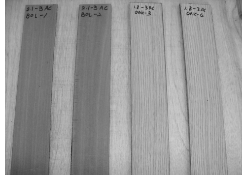
Fig. 3. Wood flooring overlaid with fancy veneer onto plywood using formulated adhesives (red: overlaid with boliva fancy veneer, white yellow: overlaid with oak fancy veneer).
