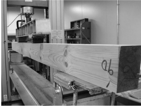
Fig. 1. Test set-up for evaluating the bending strengths of specimens (third-point loading).
