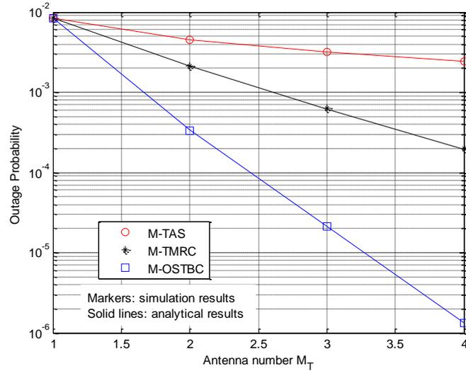
**Fig. 6.** Outage probabilities of the joint diversity schemes vs.  $M_T$ , with  $\bar{\gamma} = 10$  dB,  $K = 10$ ,  $\rho = 0.7$  and  $R = 0.5$  bps/Hz.
