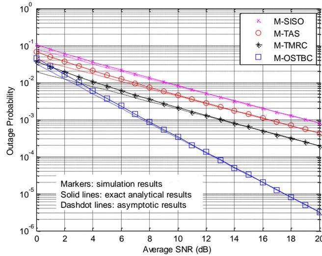
**Fig. 4.** Outage probabilities of the joint diversity schemes vs.  $\bar{\gamma}$ , with  $K = 10, M_T = 2, \rho = 0.7$  and  $R = 0.5$  bps/Hz .
