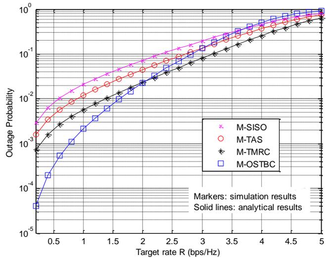
**Fig. 8.** Outage probabilities of the joint diversity schemes vs.  $R$ , with  $\bar{\gamma} = 10$  dB,  $K = 10$ ,  $M_T = 2$  and  $\rho = 0.7$ .
