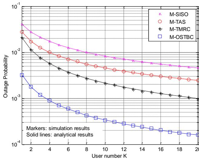
**Fig. 5.** Outage probabilities of the joint diversity schemes vs.  $K$ , with  $\bar{\gamma} = 10$  dB,  $M_T = 2, \rho = 0.7$  and  $R = 0.5$  bps/Hz .
