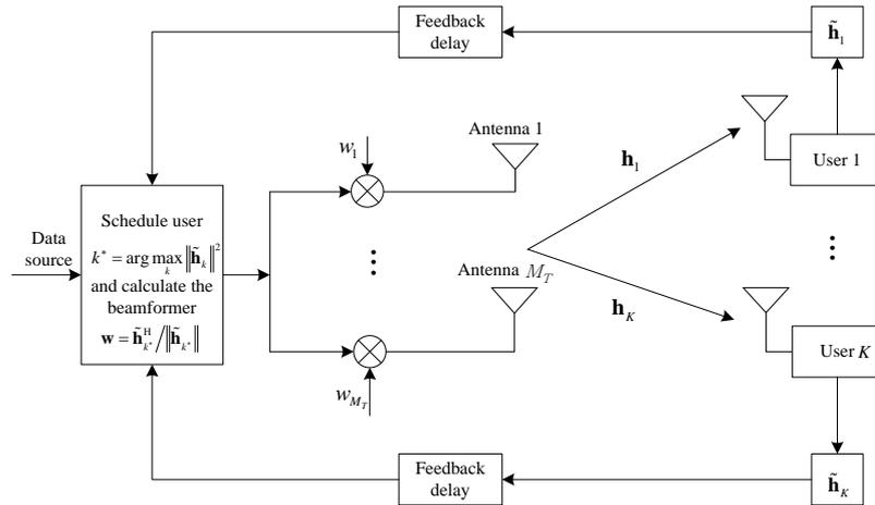
**Fig. 1.** System model of the M-TMRC scheme with outdated feedback.
