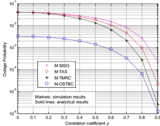
**Fig. 7.** Outage probabilities of the joint diversity schemes vs.  $\rho$ , with  $\bar{\gamma} = 10$  dB,  $K = 10$ ,  $M_T = 2$  and  $R = 0.5$  bps/Hz.
