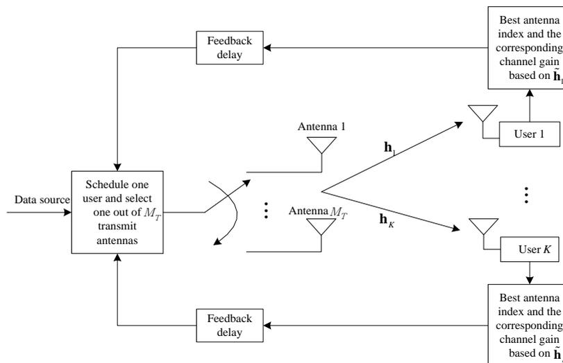
Fig. 2. System model of the M-TAS scheme with outdated feedback.
