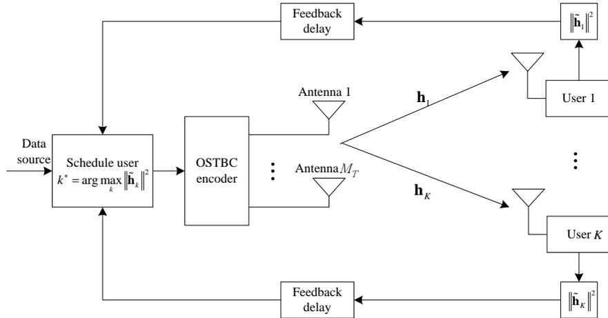
Fig. 3. System model of the M-OSTBC scheme with outdated feedback.
