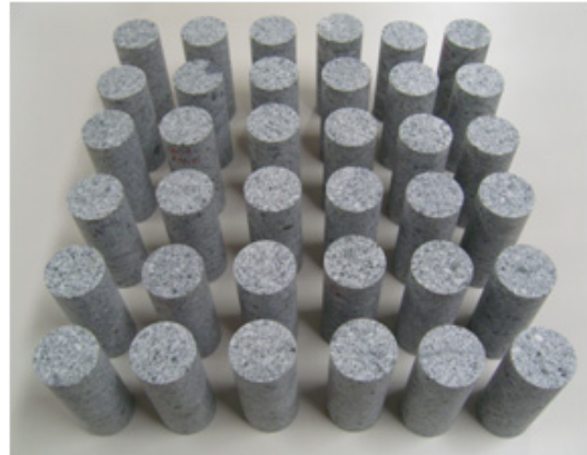
Fig. 1. Photograph of shaped granite specimens.
