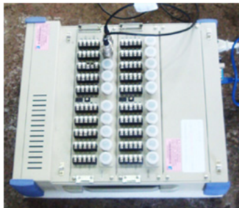
(a) 20 channel data logger
