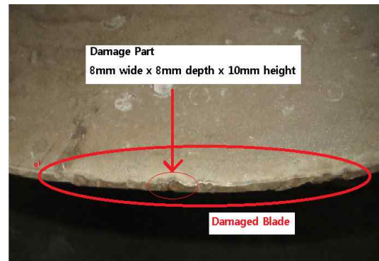
Fig. 5. Detail of Damaged Parts.
