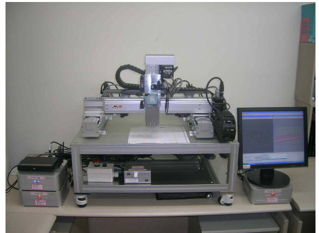
Fig. 13. Integrated prototype of automated curved hull plates forming system.
