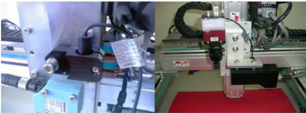
Fig. 11. Gantry robot equipped with CCD Camera, Laser Scanner, and Heating Emulation Device.
