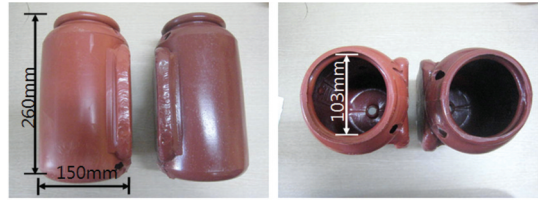
Fig. 3. Biodegradable octopus pot (Left) and PE octopus pot (Right) used in the study. Sizes are the same but biodegradable pot's color is brighter than PE pot's.
