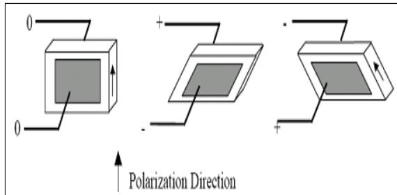
Fig. 1. Piezoelectric transformation of shear mode type.
