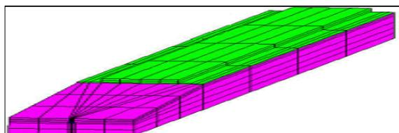
Fig. 3. Mesh division of one nozzle analysis model.
