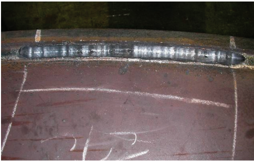
(b) Region with CO 2 gas shut off
