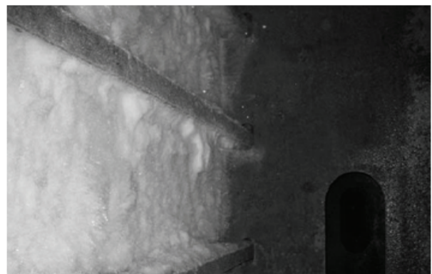
Fig. 2 Freezing of ballast water
