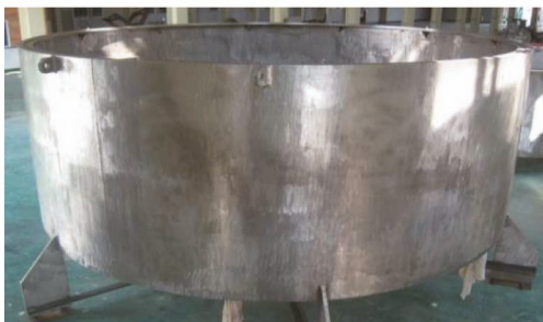
Fig. 3. Picture of Manufactured RV Mockup
