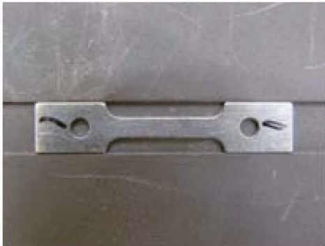
Fig. 1. Zirconium Alloy Specimens Used to Measure Mechanical Properties
