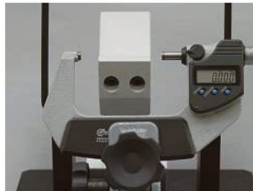
Fig. 4. Micrometer Used to Measure Irradiation Growth
